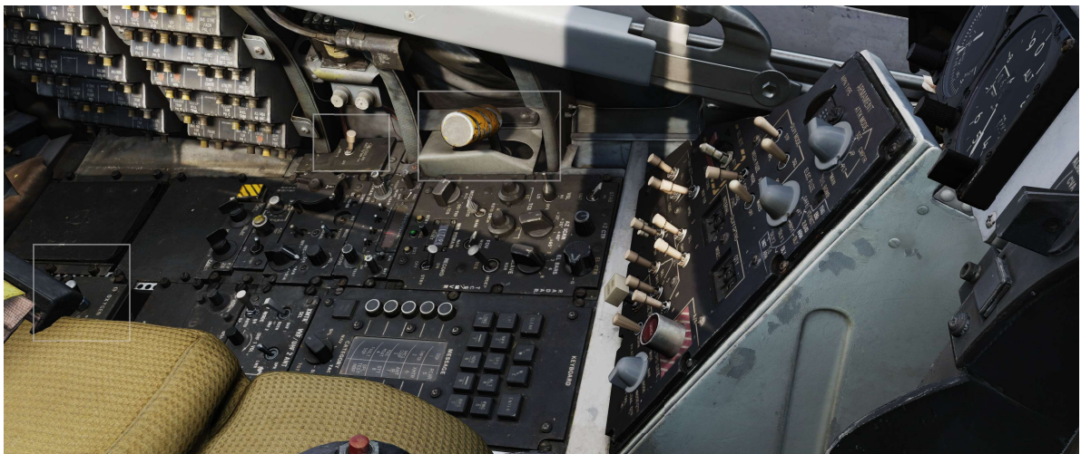
Figure 108: Left-side controls. Note the Oxygen switch, the Cooling switch and the Ejection lever.
