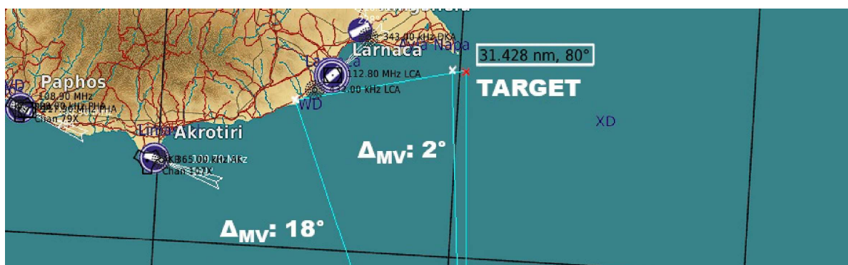
Figure 135: Example – Positional error over 100nm.
