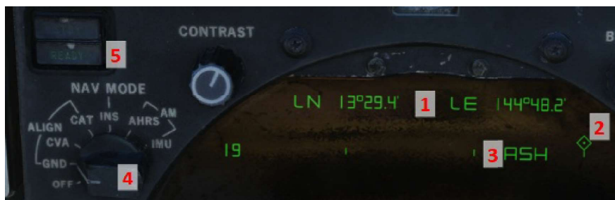
Figure 104: INS Ground alignment completed.
