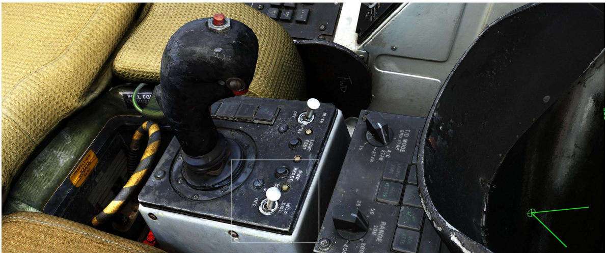
Figure 106: Detail of the HCU. Note the WCS XMIT switch.
