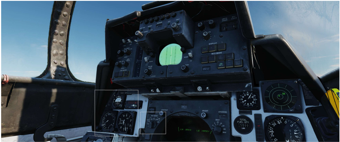
Figure 107: DDD. Highlighted are the NAV MODE knob, the barometric altimeter and the SAI.
