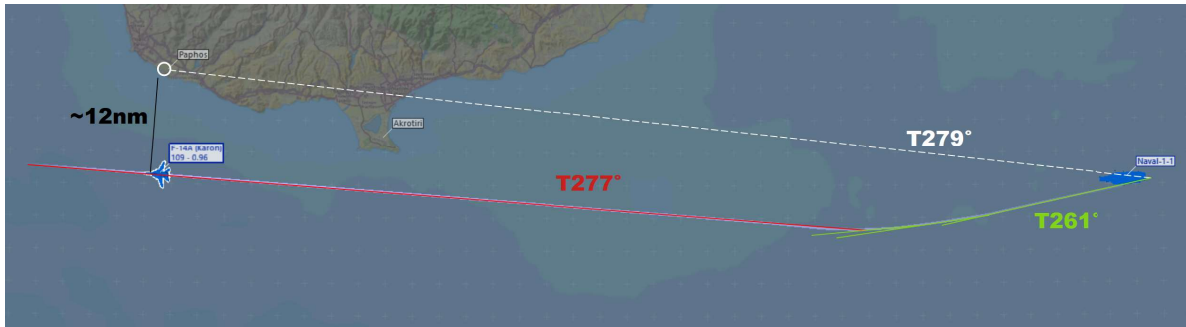
Figure 141: Non-INS navigation – AHRS re-sync: details.
